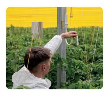
The sensor uses an infrared (IR) thermometer and adjustable arm for contactless plant leave temperature measurements. The sensor mount has two magnets for simple installation on a metallic constructions.
