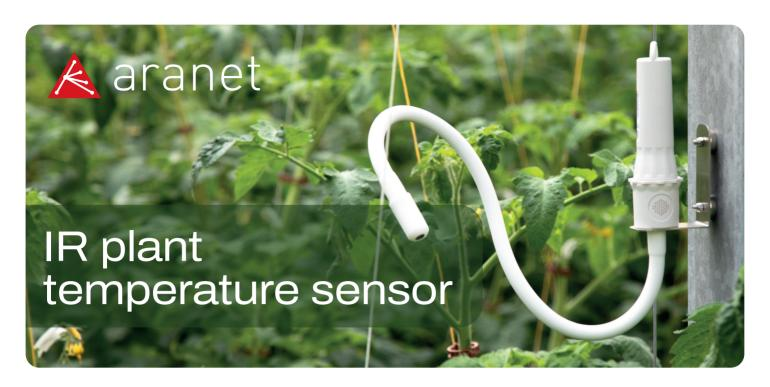
The Aranet IR Plant Temperature sensor is designed to measure the surface temperature of plant leaves. An adjustable arm provides precise sensor installation for plant temperatures measurements in greenhouse applications making it a valuable tool to calculate Vapor Pressure Deficit (VPD).
