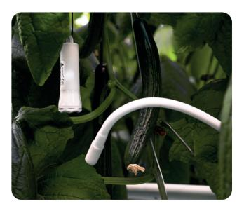
The sensor provides temperature data, which in combination with relative humidity measurements can be used to determine dew point and vapor pressure deficit.
