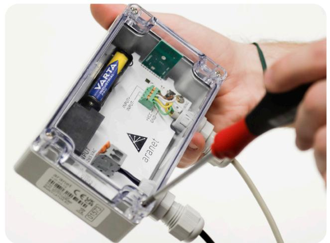
10. Screw the lid back on, and you have finished the sensor setup. Now you are ready to plug it into the power and install your sensor in your greenhouse.
