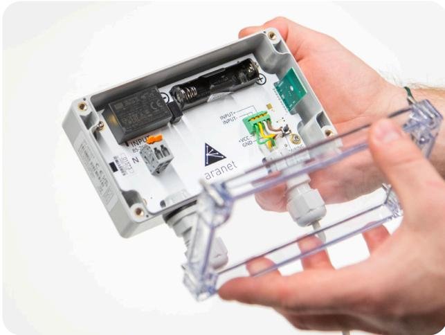
1. Unscrew and take off the transmitter's lid. Have the transmitter and 1x AA battery ready.
