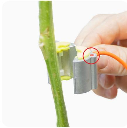
**2.** Open the sensor wide enough to place it on the stem. Make sure that the red directional mark corresponds to upward flow.
