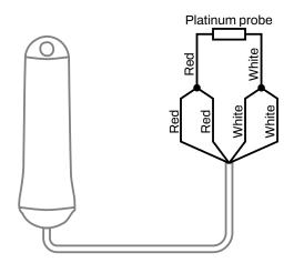
**Connecting 2-wire probe**: Connect the lead from one side of the platinum resistor to both red leads of the Aranet transmitter. Connect the lead from the other side of the platinum resistor to both white leads of the Aranet transmitter.
