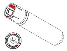
**Probe removal or installation:** To remove or install the probe, use a straight push or pull motion. Do not twist or rotate.
