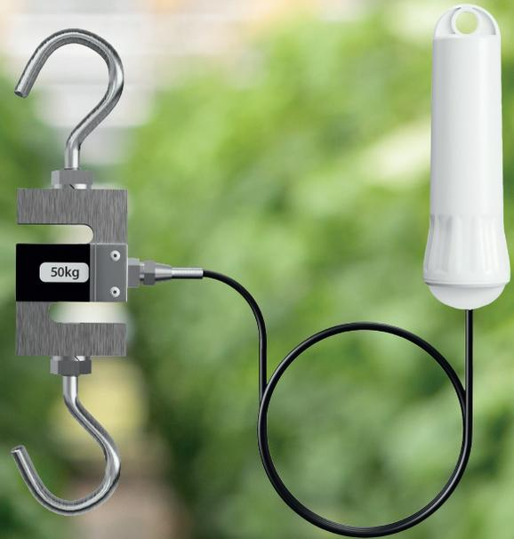
Continuous weight measurement using the [Aranet Weight sensor](#) enables real-time monitoring of various plant growth factors including biomass increase, plant weight, water addition, and drainage weight. Both the 50 kg and 100 kg versions operate wirelessly and are powered by a single AA battery. For more comprehensive insights, consider combining multiple weight sensors to detail processes within the greenhouse.
