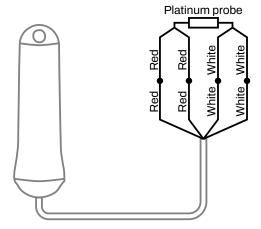
Connecting 4-wire probe: Connect one pair of leads from the platinum resistor to the red leads on the Aranet transmitter. Connect the other pair of leads from the platinum resistor to the white leads on the Aranet transmitter.
