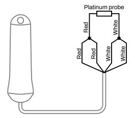
Connecting 2-wire probe: Connect the lead from one side of the platinum resistor to both red leads of the Aranet transmitter. Connect the lead from the other side of the platinum resistor to both white leads of the Aranet transmitter.
