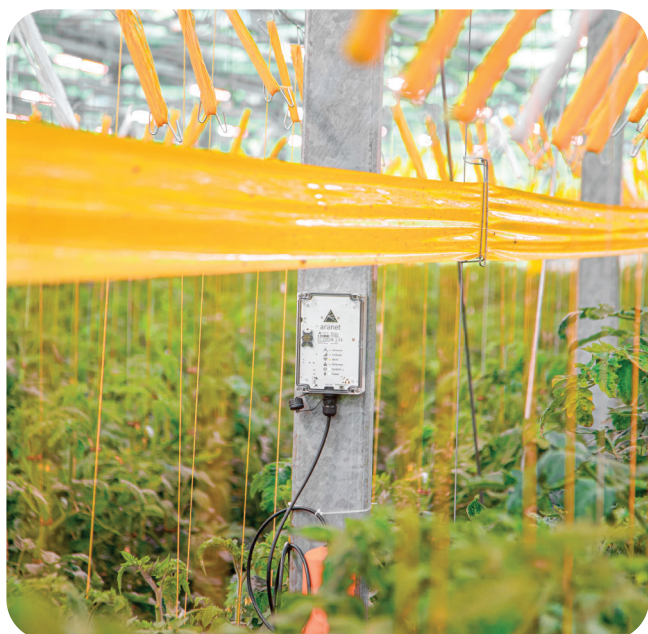
Example of the Base station installed above the tomato plants in the greenhouse.
