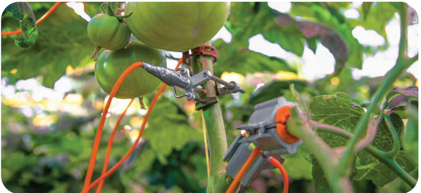
Example of a reference plant in the greenhouse equipped with SAP flow sensors to study flow in both stem directions, along with a Stem Diameter sensor.
