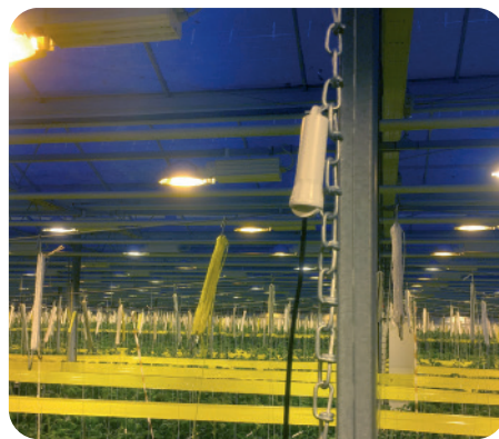
If the sensor has an extended wire, position the transmitter (white body) above the plants.
