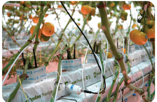
Installation example of WET150 sensor with sensor holder installed in the tomato greenhouse.
