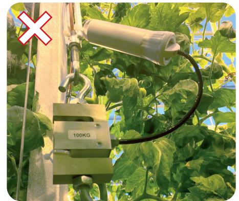
It is recommended not to position the sensor transmitter (white body) surrounded by leaves.
