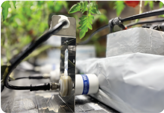
WET150 sensor equipped with an installation bracket for monitoring VWC, EC, and temperature in substrate
