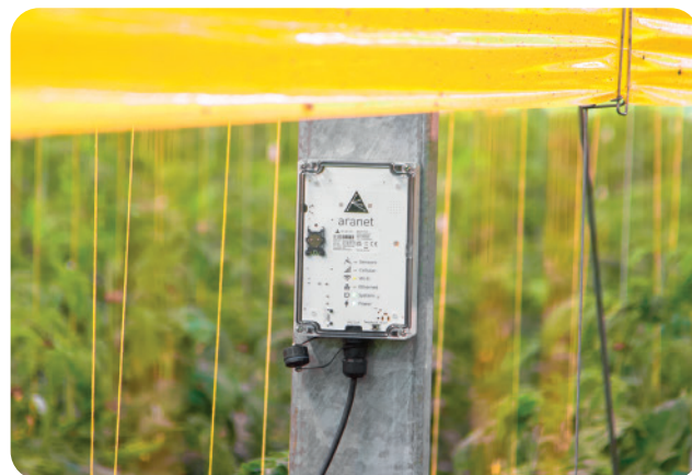
Example of wireless sensor and base station installed in the greenhouse.
