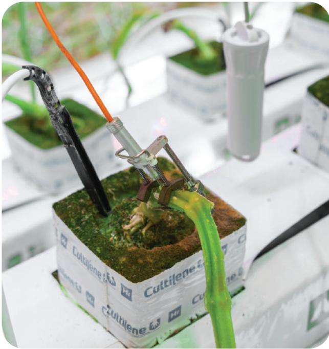
Example of Stem Diameter sensor installed in the greenhouse
