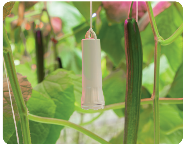
T/RH sensor installed in the greenhouse.
