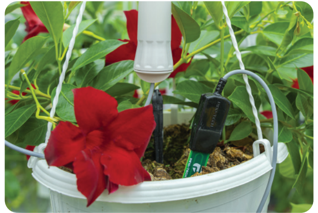
Example of Soil Moisture sensor installation.
