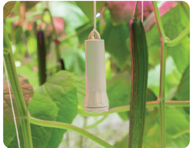
T/RH sensor installed in the greenhouse.
