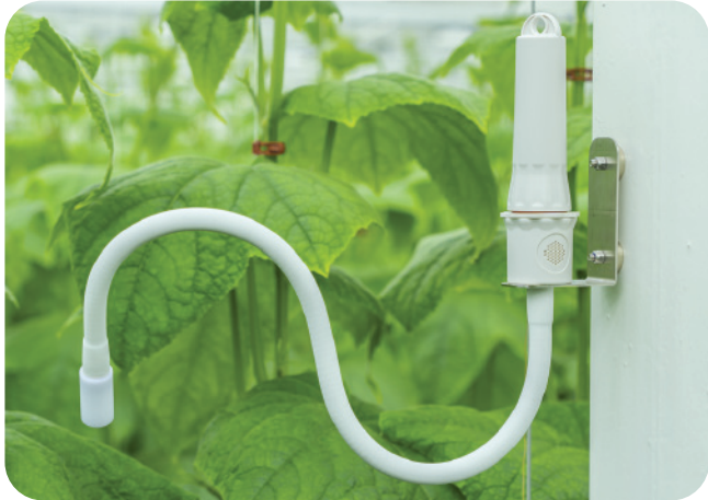
IR Plant Temperature sensor installed in the greenhouse.
