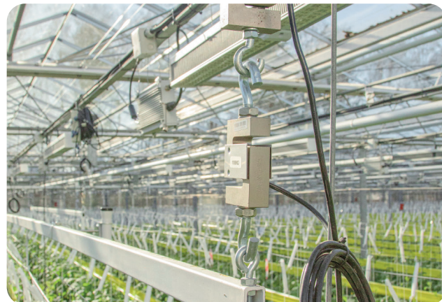
Example of using a Weight sensor with a frame for plant growth monitoring.
