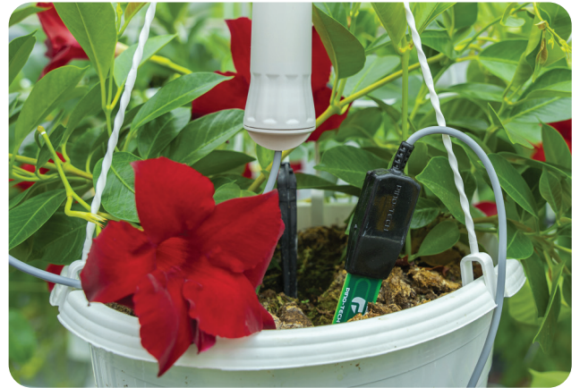
Example of Soil Moisture sensor installation.
