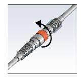
**Step 2:** Use your fingers to securely tighten the locking nut until it is snug.
