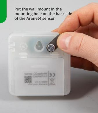
Push the wall mount upwards in a locked position
